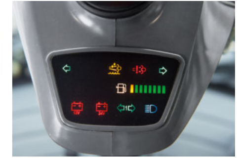
The central indicator lights on the steering column provide information about the most important driving parameters.
