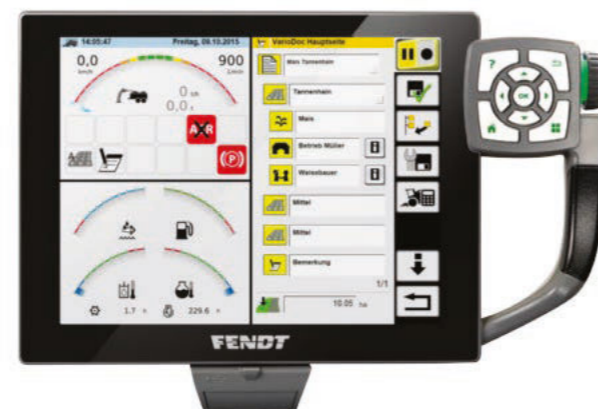
The Fendt documentation system VarioDoc logs all relevant data during operation.
