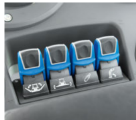
Functions such as open/close maize header and pick-up support wheels, header tilt, lift/lower discharge chute are conveniently controlled using the toggle switches.
