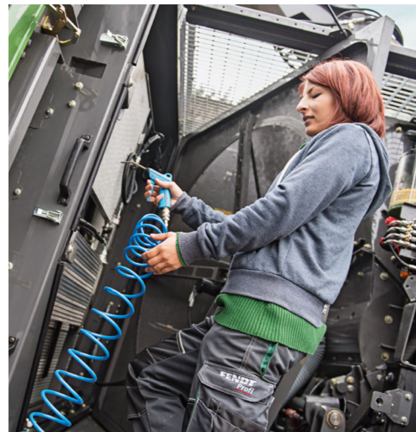
The components on the Katana are especially easy to access thanks to large maintenance flaps, which open upwards, not sideways. The maintenance lighting makes all the difference in the dark.
