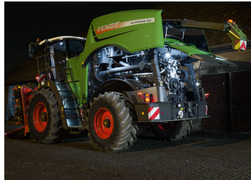
Best working conditions in the dark thanks to optional LED maintenance lighting.
