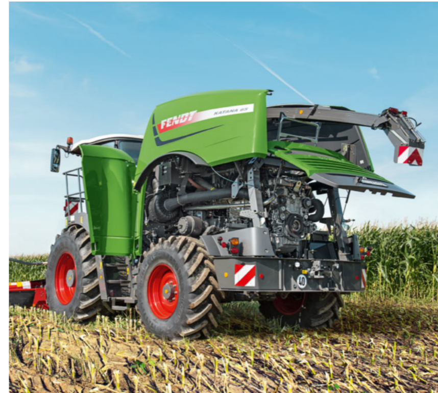
Easily accessible storage and battery compartments at the rear of the vehicle offer plenty of space, for example for the optional toolbox.
