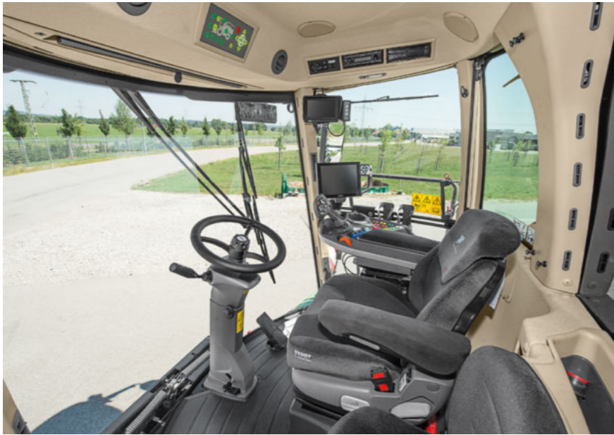
The Visio5 cab has been designed for optimum visibility and offers perfect ergonomics and easy-to-use controls in the workplace. Thanks to the special shape of the roof line, operators always have the chute flap in view. Automatic climate control and heating guarantee a pleasant working environment.
